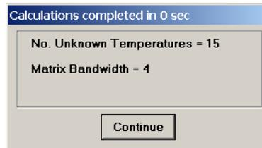
Click the Continue button. A number of the output display windows in the **View** menu will now be accessible. The temperatures within the wall can be displayed at each node by selecting **Temperatures** from the **View** menu. Press and hold the left mouse down and move it within the outline. The temperature at the cursor location will be displayed in the status bar at the upper left of the screen, replacing the cursor coordinates.
